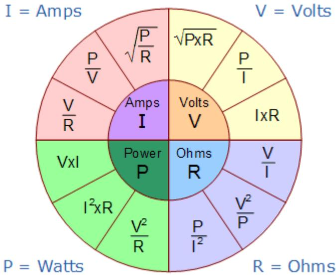
As well as using the *Ohm's Law Pie Chart* shown above, we can also put the individual Ohm's Law equations into a simple matrix table as shown for easy reference when calculating an unknown value.
