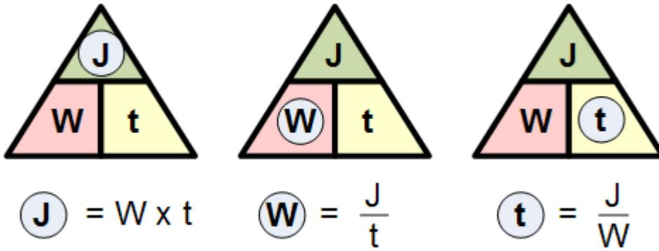
We said previously that electrical energy is defined as being watts per second or *joules*. Although electrical energy is measured in Joules it can become a very large value when used to calculate the energy consumed by a component.
