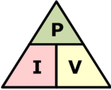
and again, transposing the basic Ohms Law equation above for power gives us the following combinations of the same equation to find the various individual quantities:
